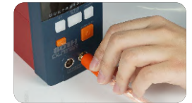
③ Insert the mobile welding pen and make sure the connection is solid.
